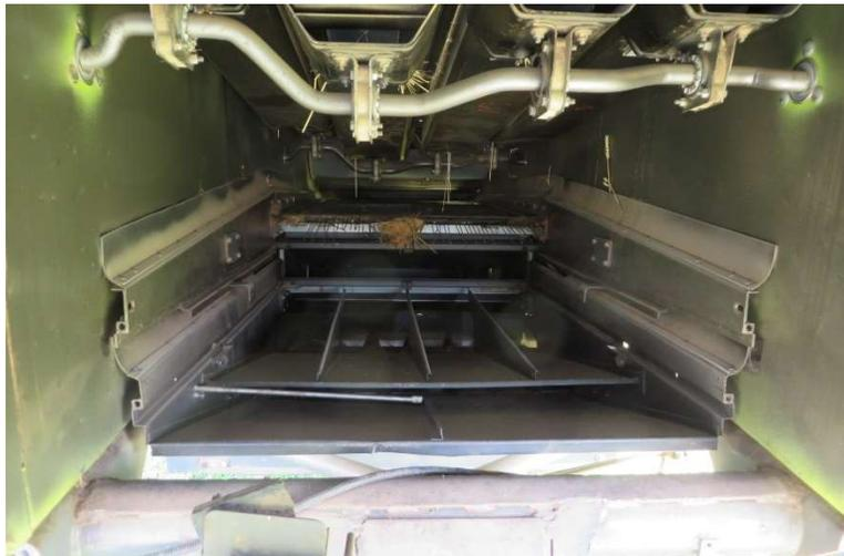
*Fig. 9. Back End of Claas Combine with Screen Missing to Allow Additional Chaff be Included with Grain, Inflating the Number of Bags Harvested to Increase Income but burdening Farmers with Extra Winnowing Work.*
