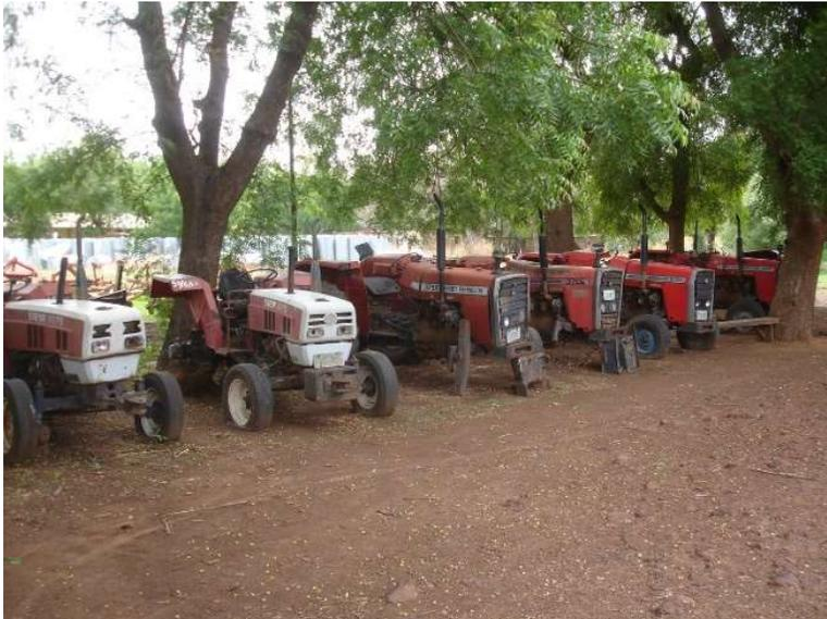
*Fig. 7. Line of government owned and operated tractor at Nigerian Agriculture Development Project, surveyed out of use with well less than the 10,000 hours designed work live, often with the odometer vandalized.*
