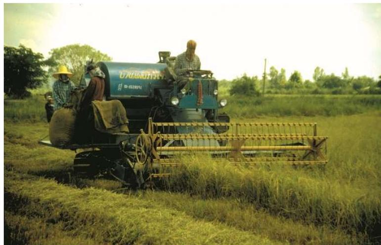
*Fig. 5. Small rice combine used in Thailand that will harvest 1 rai (1/6<sup>th</sup> ha.) in an hour and allow further crop intensification to 5 paddy crops in 2 years.*
