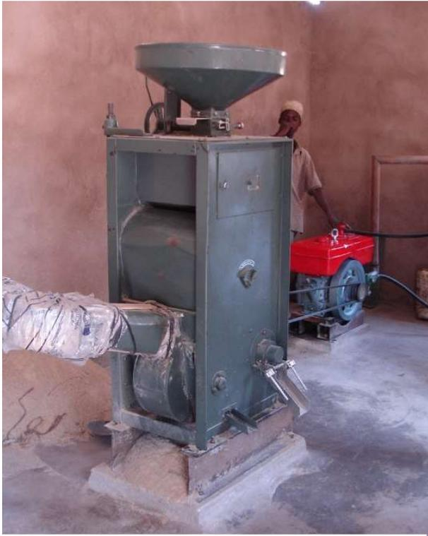
Fig. 16. Also, individuals invested in additional grain mills like this 2-stage rice mill.
