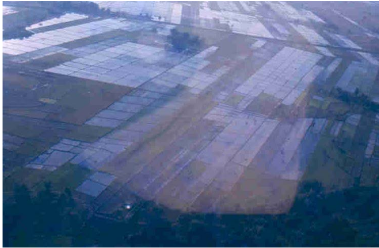
Photo 8.5 Aerial view of rice irrigation in Central Luzon Philippines showing long narrow fields running from canal to drain minimizing coordination needs between farmers.
