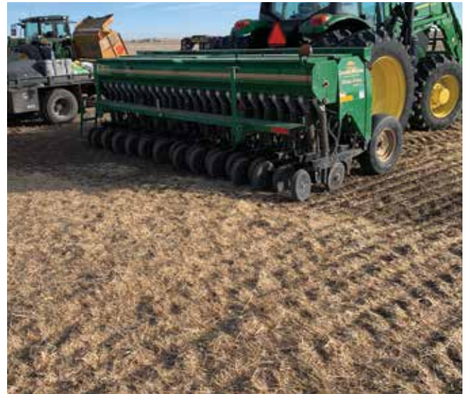
A no-till seed drill can be used to overseed existing pastures or seed reclamation projects.
